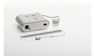
The FITBONE® System consists of an intramedullary lengthening nail, a receiver and an external control set.
