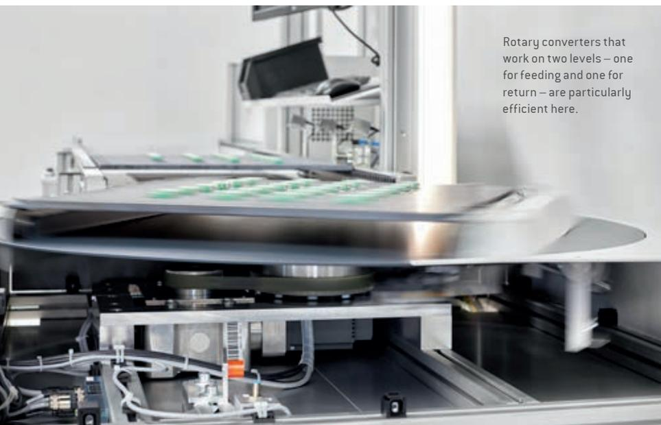
Rotary converters that work on two levels – one for feeding and one for return – are particularly efficient here.
