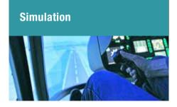
Flight simulators enhance air safety. They can be used to provide civilian and military pilots with practical instruction and training. Control loading systems are the sensitive humanmachine interfaces in such simulators. We offer our customers these systems from a single source, including all the integrated hardware and peripherals as well as the necessary software systems and programming for aircraft type-specific databases.
