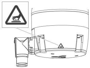
There is a safety sign on the servo actuator housing that warns against hot surfaces. This safety sign may **not** be removed.
