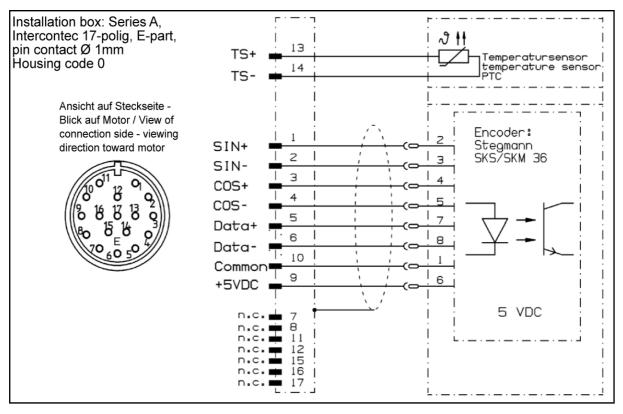
Option "E" and "V" with 560 V intermediate voltage —signal (pin assignment 5)
