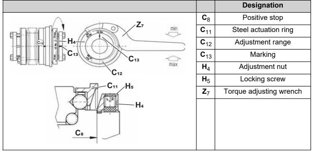
Tbl-7: Disengaging torque setting
