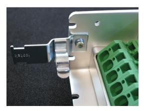
In order to maintain conformity with the EMC limit values and ensure the functioning of the drive amplifier the shielding of the motor cable must be connected to the housing of the drive amplifier with low impedance and over a large area.
