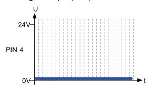
A permanent and continuous low signal (0 V) at PIN 4 indicates that the lubricator is ready for operation and that there are no active errors. The lubricator operates according to the settings made and delivers lubricant from the cartridge to the outlet accordingly.
