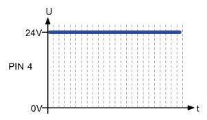
A permanent and continuous high signal (+24 V) at PIN 4 indicates that there is an active error. The error must be read on the display of the lubricator (see chapter 6.4 "Error messages"). The lubricator does not deliver any lubricant!
