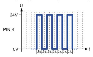
Use of the output signal 0.5 Hz is independent of inversion of the output signals. In advanced programming, the empty cartridge signal L must be changed from the parameter value L1 to L2.
