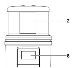
The final position is reached after two full turns when the label of the lubricant cartridge [2] is aligned flush with the front cover [8] of the lubricator.
