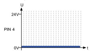
A permanent and continuous low signal (0 V) at PIN 4 indicates that there is **no** active error.
