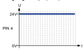
A permanent and continuous high signal (+24 V) at PIN 4 indicates that there is **one** active error.
