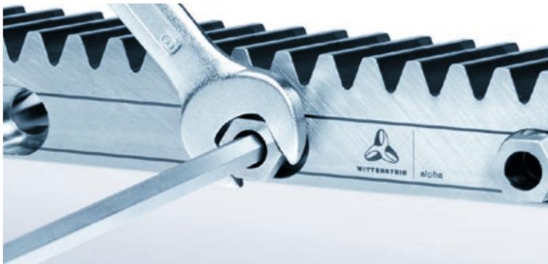
Previously, enormous effort was required to clamp racks to the mounting base using screw clamps. INIRA® clamping integrates the clamping device in the rack. The rack incorporates a mounting sleeve which is guided over the head of the fastening screw to ensure quick and ergonomic clamping.
