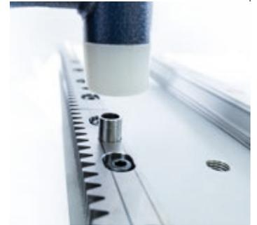
The assembly bushing is then driven in flush using a hammer.
