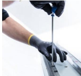
The assembly bushing and the assembly pin are turned in opposite directions until the bushing engages in the pin bore and then pushed in by hand up to the second marking.
