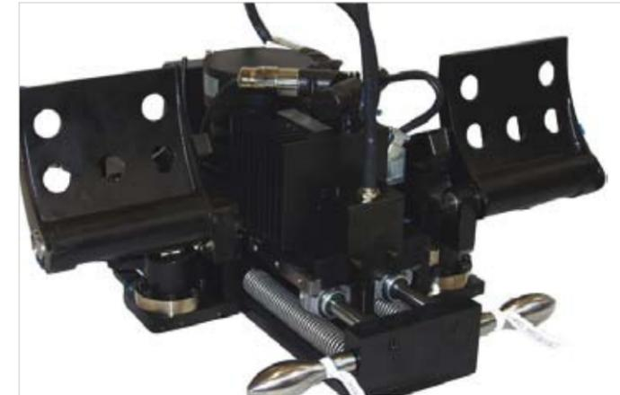
The active rudder pedal assembly is a combination of one integrated control loading actuator consisting of motor, gearbox and electronics, force sensors and pedal arrangement. The pedal arrangement can provide linear or rotary motion of the pedals and integrated toe brakes.
