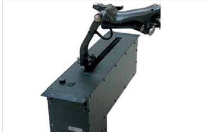
The active linear and rotary throttles are a combination of a single control loading actuator with linear or rotary gearing, electronics and force sensor. Dual throttle variants are also available.
