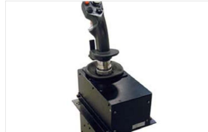
The sidestick has integrated motors, gearboxes, control loading electronics and force sensor technology.
