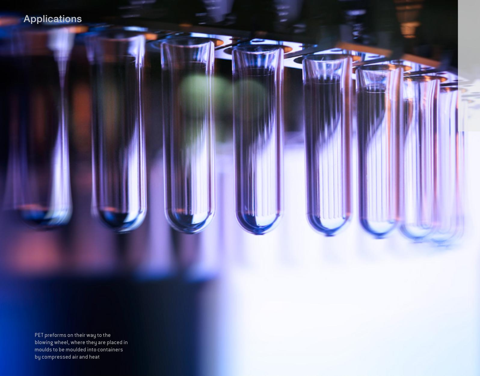
PET preforms on their way to the blowing wheel, where they are placed in moulds to be moulded into containers by compressed air and heat
