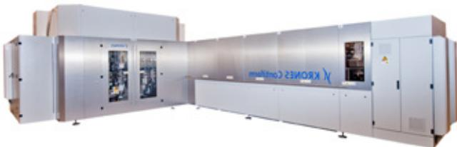
The stretch blow moulders in the Krones Contiform 3 series impress with up to 81,000 PET bottles per hour.
