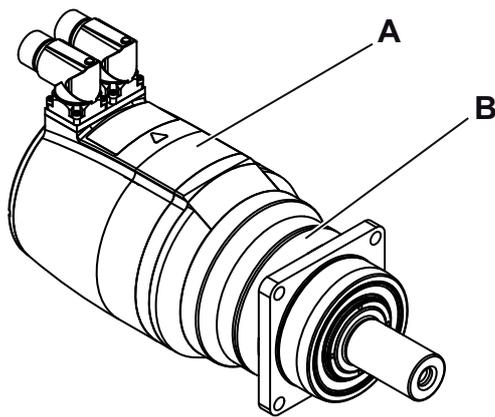
The servo actuator is a combination of a low-backlash planetary gearbox (B) and an AC servomotor (A).
