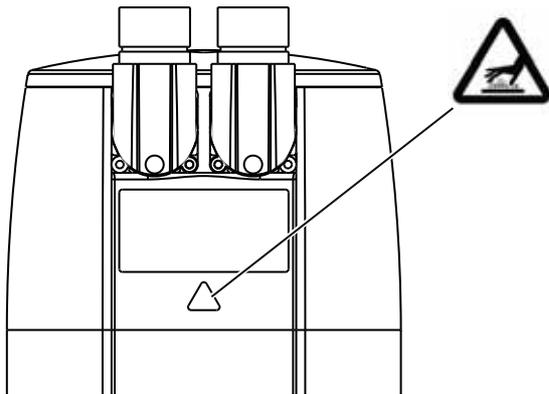
There is a safety sign on the servo actuator housing that warns against hot surfaces. This safety sign may **not** be removed.
