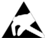
Component sensitive to electrostatic discharge
